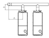
The common flue way is made of INOX 316L.
