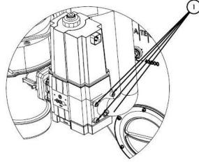
Loosen the four bolts from the gas valve as shown in figure (1).
