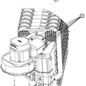
Then remove the 4 bolts from the burnerhood as shown in figure (2).
