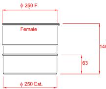
Inox adaptor between T-piece and aluminum flue-gas connection to the boiler:
