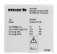
Due to pressure difference between flue gas outlet - and combustion air inlet pipe the minimum heat input is defined:
